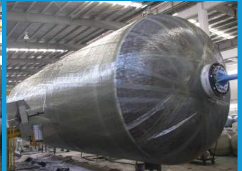
Computer Controlled Filament Winding
